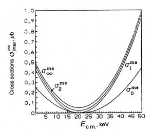
FIG. 24. Contributions  $\sigma_{j_{\max}}^{ms}$ ,  $j_{\max}=0,1,2$ , to the magnetic-nuclear total cross section  $\sigma_{\infty}^{ms}$  for triplet nn scattering.
