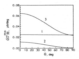
FIG. 22. Magnetic-nuclear differential cross section  $d\sigma^{ms}(\theta)$  for triplet nn scattering at 5, 20, and 40 keV (curves 1, 2, and 3, respectively).
