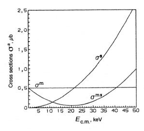
FIG. 23. Magnetic  $\sigma^m$ , nuclear  $\sigma^s$ , and magnetic-nuclear  $\sigma^{ms}$  total cross sections for triplet nn scattering.
