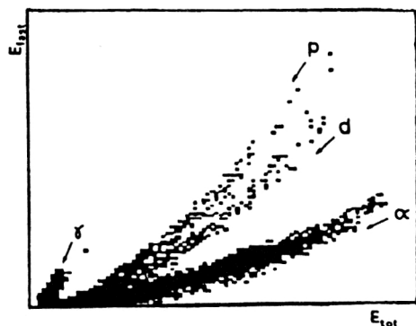
FIG. 19. Two-dimensional E_{fast}-E_{tot} spectrum (Ref. 99).
